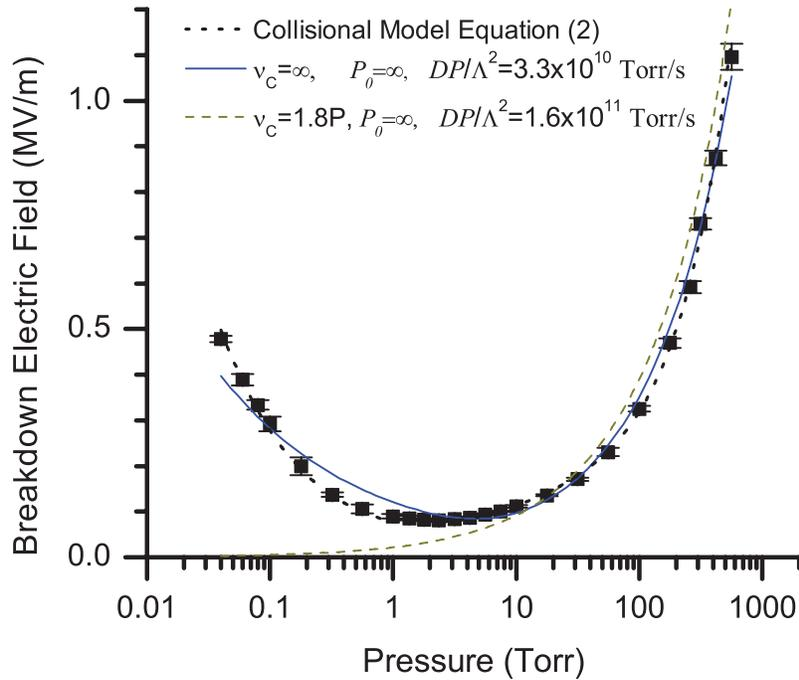
FIG. 3. Threshold breakdown electric field for a 500  $\mu\text{m}$  gap at 1.7 GHz. The pressure regions for breakdown inside (high pressures) and outside (low pressures) the gap overlap, and the data are better modeled as two simultaneous breakdown processes using Equation (2).
