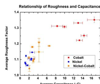
**Figure 4.** The cobalt samples have the highest roughness factors. The nickel-cobalt samples seem to be more related with the nickel samples from a roughness standpoint.
