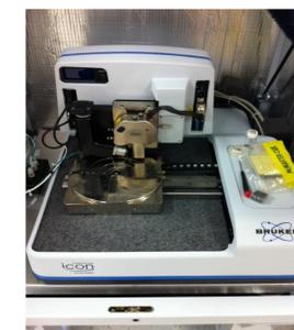
**Figure 6.** AFM used for roughness characterization. The model is the Bruker, Dimension Icon .
