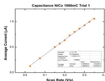
**Figure 2.** Plot of the average current and scan rate. The slope of this linear trend is the capacitance value for one trial on a given sample, the NiCo 1000mC sample in this example.
