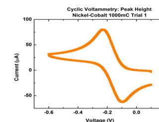
**Figure 7.** Cyclic voltammogram using 5mM hexaamineruthenium (III) chloride and 1M potassium chloride as the electrolyte. Example of a "duck curve" for peak height to be measured.
