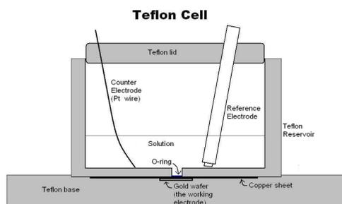
**Figure 1.** Rendering of the custom Teflon cell for electrochemical measurements and fabrication of samples.
