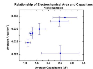
**Figure 5.** The nickel samples seem to have a linear trend for area and capacitance. This capacitance was done with 1M sodium hydroxide.
