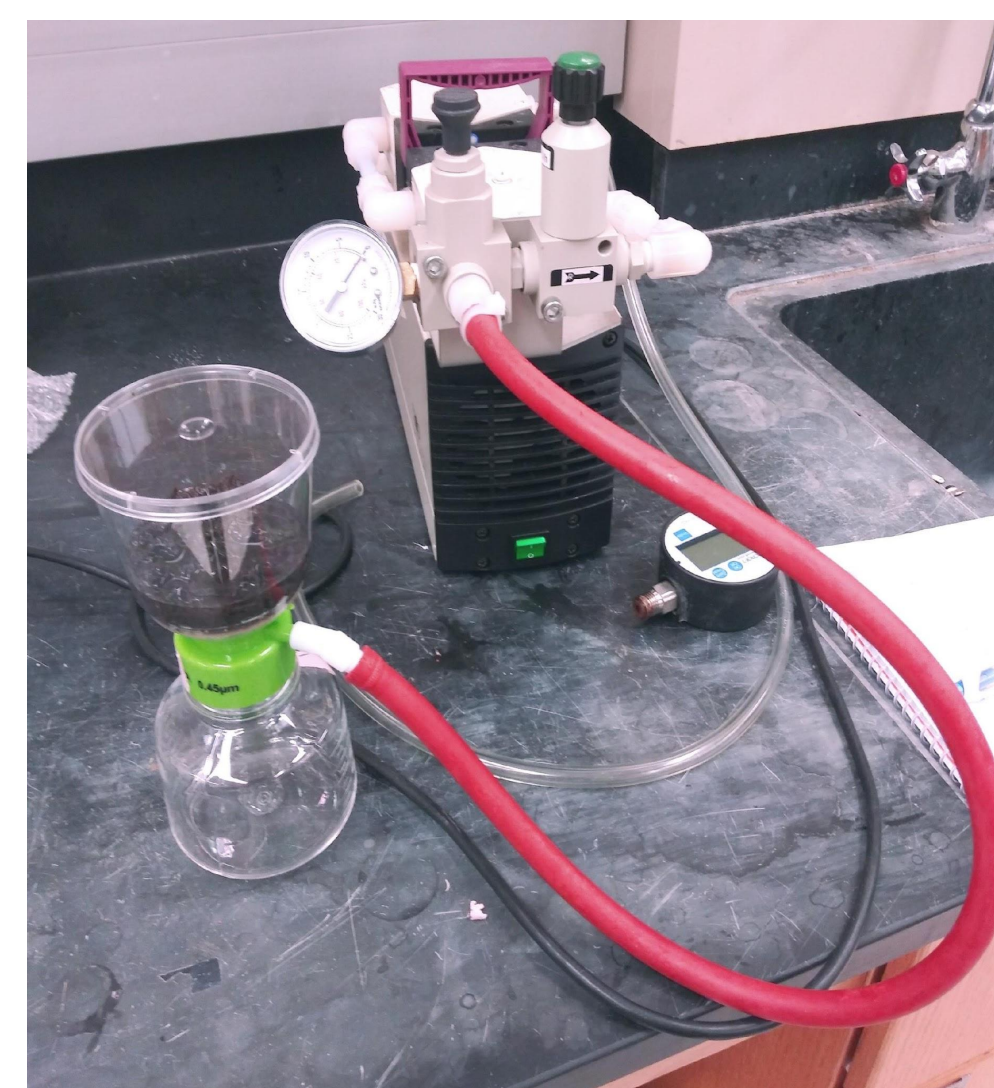
Microlysimeter (green) with peat core attached to vacuum set to 70 kPa.
