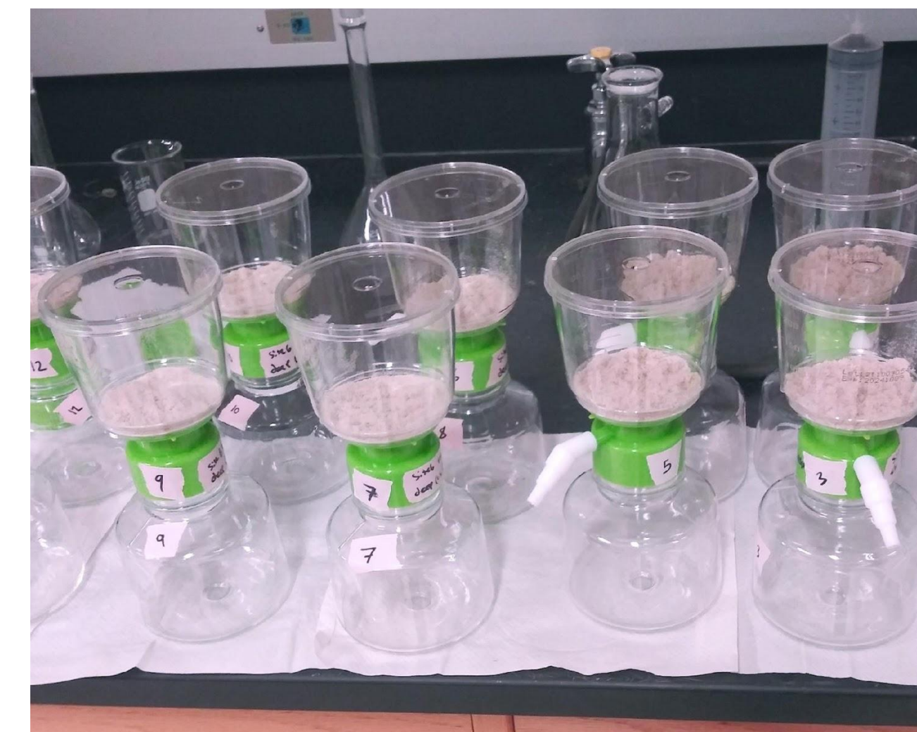
8 microlysimeters with 20 g of sand added before peat was added to reduce clogging
