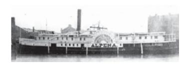
She had a pilothouse forward, strengthening arches along each side, and a single stack forward of the engine. When the wreck of the *Alpena* finally is found, it will be these distinctive paddlewheels and the vertical beam engine that will enable researchers to identify her.
