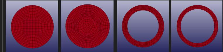
Coarse mesh solid (36800 elements)      Fine Mesh Solid (92850 elements)      0.8 mm Hollow      0.6 mm Hollow
