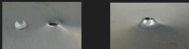
Plugging Failure      Petaling Failure
