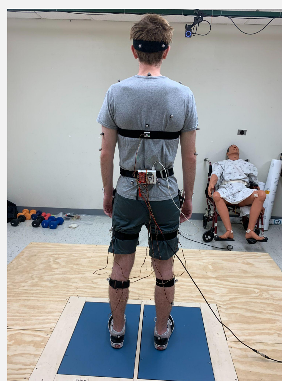
fig. 1: IMU, force plate, and markers setup
