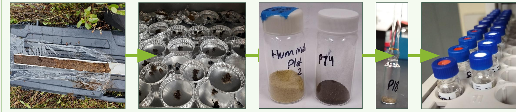
Fig. 2 Processing of peat samples from left to right: peat core in the field, samples drying in oven, ground peat sample, processed HPLC samples.
