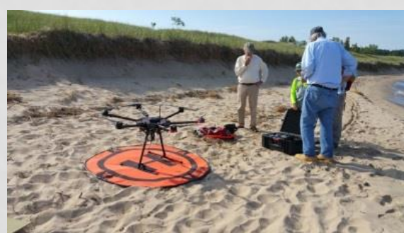
Figure 2: The DJI Matrice M200 drone carrying the RGB DJI X5S aerial camera flown on March 17 th 2018.
