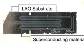
Photograph of the test sample. The control sample has the same layout and dimensions.
