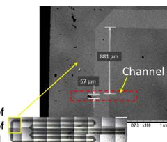
Polarized light microscope image of the test sample. The channel of columnar defects is highlighted.
