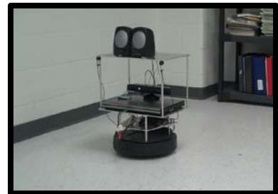
Prototype of the Mobile System for Echolocation Data-collection
